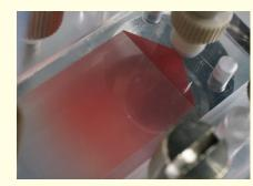
■ The polymer CTC chip was developed to selectively capture cancer cells by combining a microfluidic device with an antigen-antibody reaction. The chip is equipped with many fine posts, whose surfaces are coated with antibodies that bind to antigens specific to the cancer cells. This allows only cancer cells to be selectively captured on the surface from the sample flowing through the chip.
